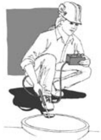
*Test the oxygen content in the air with an oxygen monitor before you enter a confined space.*
